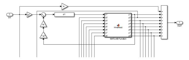
The diagram shows only the first delay line. Imagine another seven delay lines being repeated in the diagram but each delay line has an individual delay and associated feedback gain block. The Householder reflection (i.e. hhreflect function) is essentially mixing/permuting the signals without changing the energy of the total signal. Therefore, we are essentially duplicating the incoming signal and feeding it back with small time displacements. The result is a reverberation effect.
